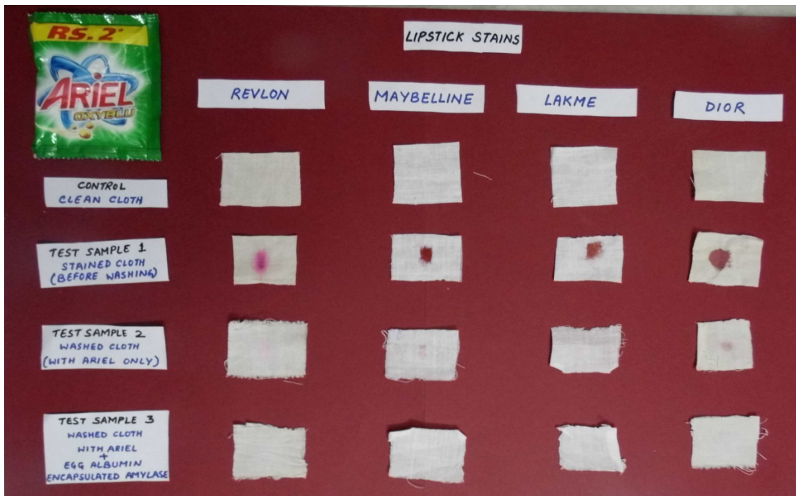
Figure 4 Washing results of stained cloth pieces with Ariel only and Ariel with Vigna mungo amylase bound chemically modified egg albumin bio-active micropreparation
